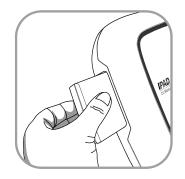
2. Insert a new battery pack in the direction of the arrow with the label facing upward as shown in the figure below.
